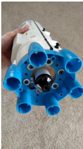
Custom retaining bracket for the motor: Expecting to fly with an Aerotech F50 ~ so far so good!
