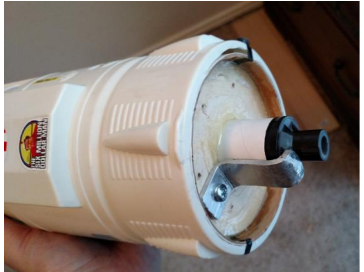
So after a lot of thought on fins, I decided to go with removable fins. I'm trying to keep as close as possible to the original toy design; adding removable fins allows me to maintain the original form factor outside of flying. Found some fins that work however I had to sacrifice another kit. Used the 3D printer to print fin mounts:
